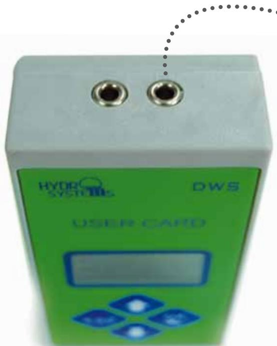
The device will operate effectively within a temperature range from -10 °C to +70 °C.
